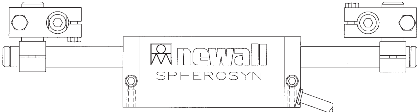
Scale Supports Inverted
