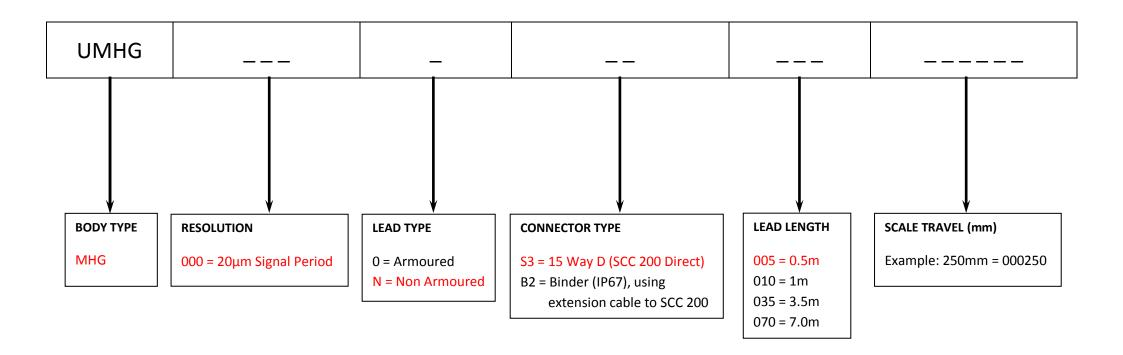
THIS ENCODER CAN ONLY BE USED WITH THE SCC 200 MODULE SUPPLIED
